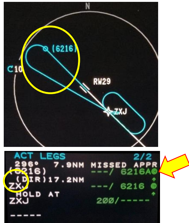
Figure 2b. After the crew uses the left FMS to activate Temperature Compensation, the “R” turn to ZXJ is initially removed (blacked) on the right FMS and will subsequently be removed on both FMSs. The map display may differ from this example.
