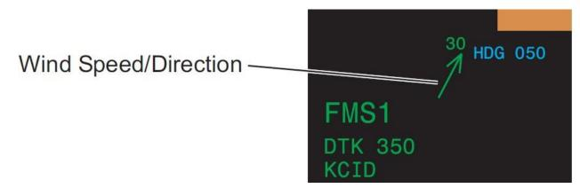
Wind magnitude and direction is shown full-time to the left of the heading readout on the PFD. Wind magnitude and direction is shown to the left of the heading readout on the MFD Rose, Arc, and PPOS Map display formats.
