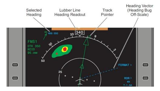
The track or drift angle is the (wind correction angle) or the angle the aircraft needs to fly into the wind to maintain a straight course over the ground. In the above example you can use the following numbers:
