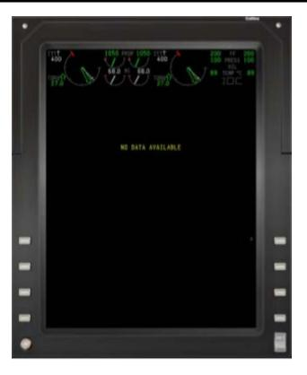
Dropping of MDT Tables and Checklist Another effect of battery depletion is the Non-Volatile Memory items, namely the Maintenance Diagnostic Tables (MDT) and the aircraft checklist files will be erased. This can be easily seen when attempting to enter the Maintenance Main Menu pages with a dead battery. The prompt No Data Available will be seen on the screen.
