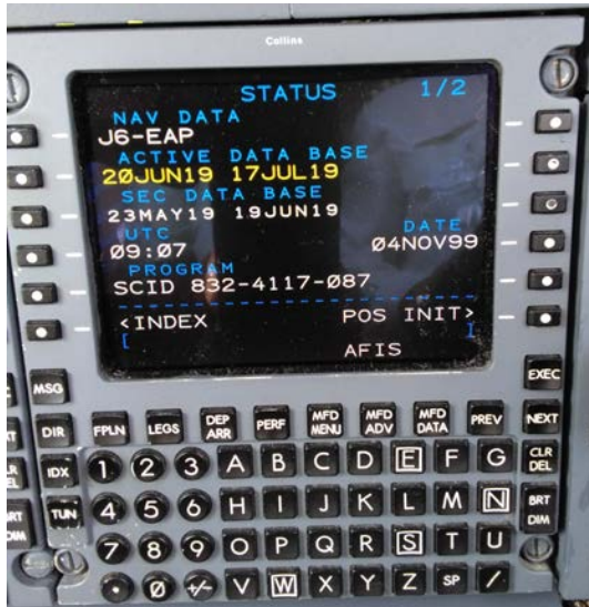
Figure 1. Example of FMS battery failure as shown on a Collins Aerospace Control Display Unit.
