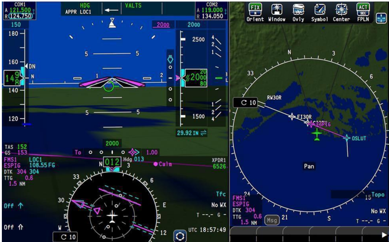
Figure 3. Approach armed after FMS flight plan is cleaned up to inbound course.
