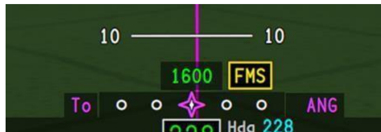
Figure 4. FMS Comparator Failure Message.
