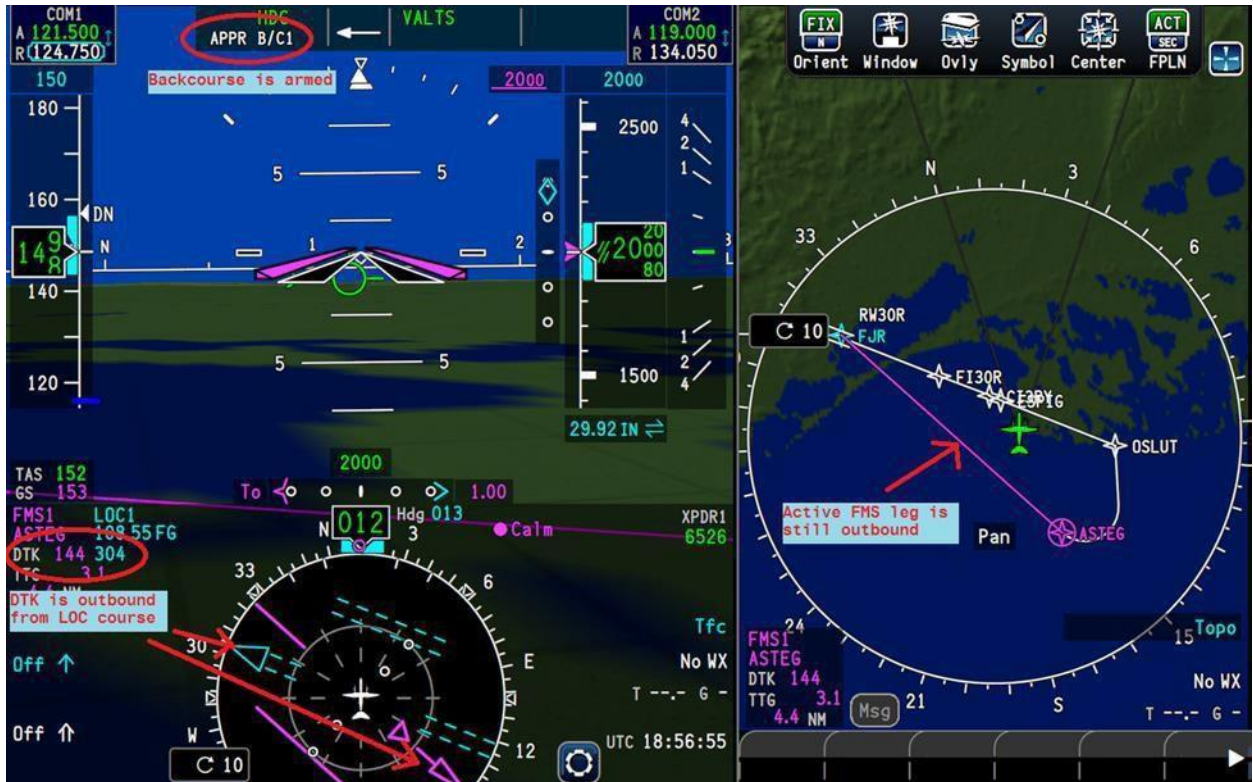
Figure 2. FMS outbound active leg with approach armed.
