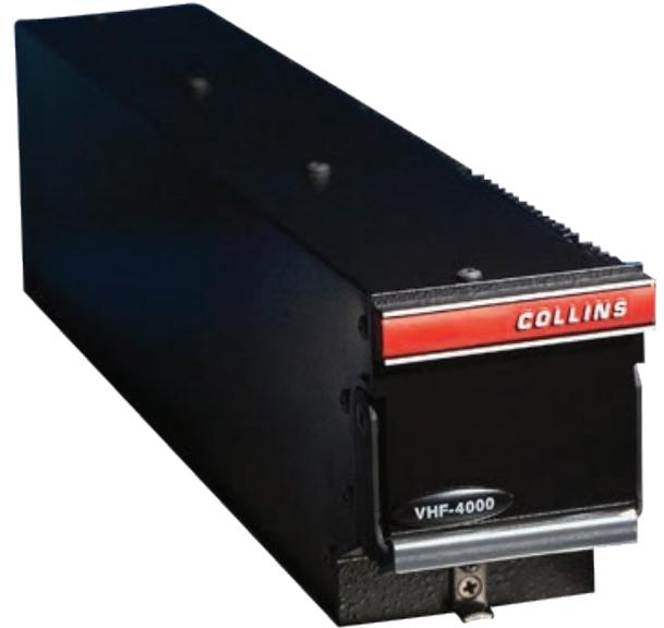
*Rockwell Collins offers a new series of VHF-4000(E) part numbers as form and fit replacements to the current part number series that will be discontinued.*
