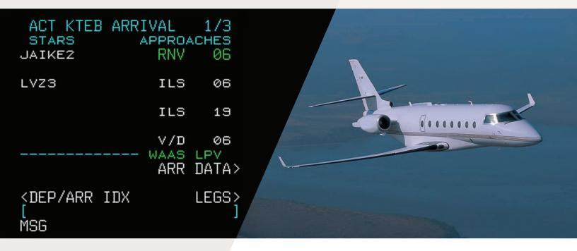
LPV will provide pilots unprecedented access to runways and airports that have not deployed an ILS approach.
