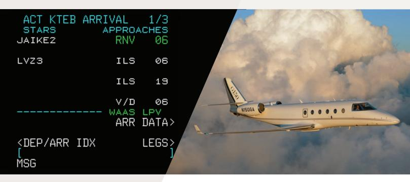
LPV will provide pilots unprecedented access to runways and airports that have not deployed an ILS approach. With an LPV upgrade for your Pro Line 21 equipped Gulfstream G150 you have increased flexibility to land more places, more often by accessing lower LPV Decision Altitudes on RNAV instrument approaches. LPV minimums as low as 200 feet with ½ mile of visibility are now published on RNAV approach charts and the flight deck operation is very similar to Category I ILS approaches.
