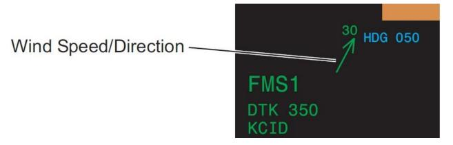
Wind magnitude and direction is shown full-time to the left of the heading readout on the PFD. Wind magnitude and direction is shown to the left of the heading readout on the MFD Rose, Arc, and PPOS Map display formats.
