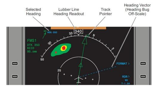
The track or drift angle is the (wind correction angle) or the angle the aircraft needs to fly into the wind to maintain a straight course over the ground.
