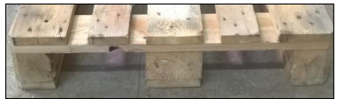
4) Pallet accessible at the front end (min. 10 cm clearance height)
