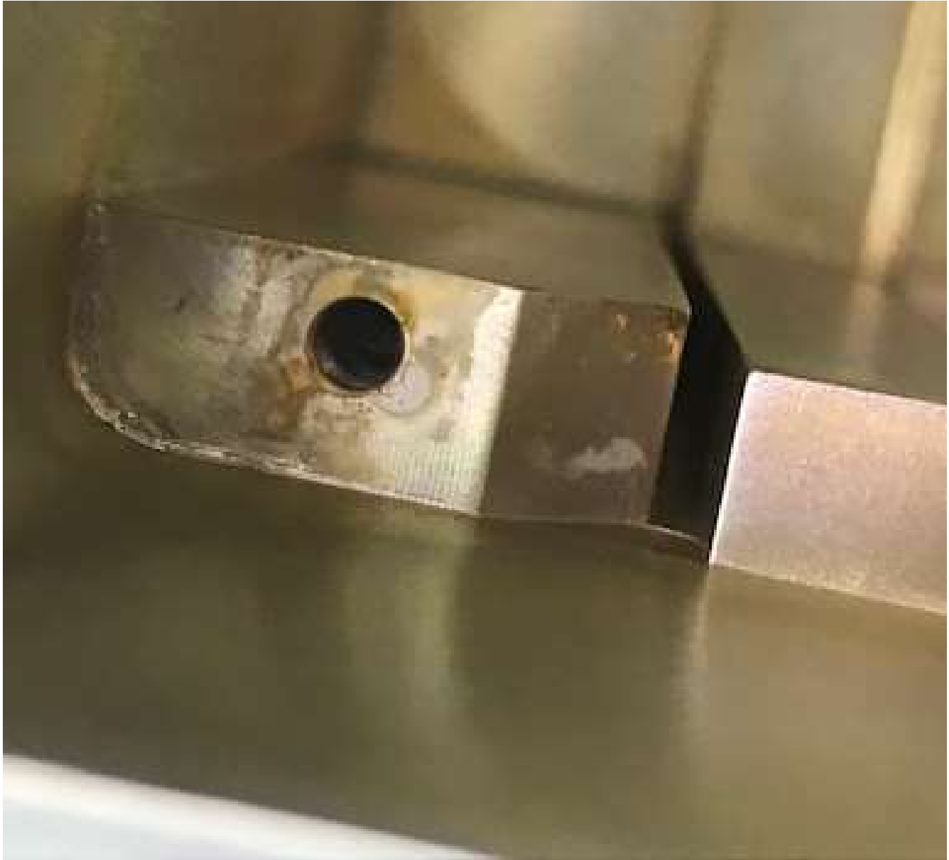
Figure 11: This is representative of either chemical conversion coating or deoxidizer splatter and is common around holes.
