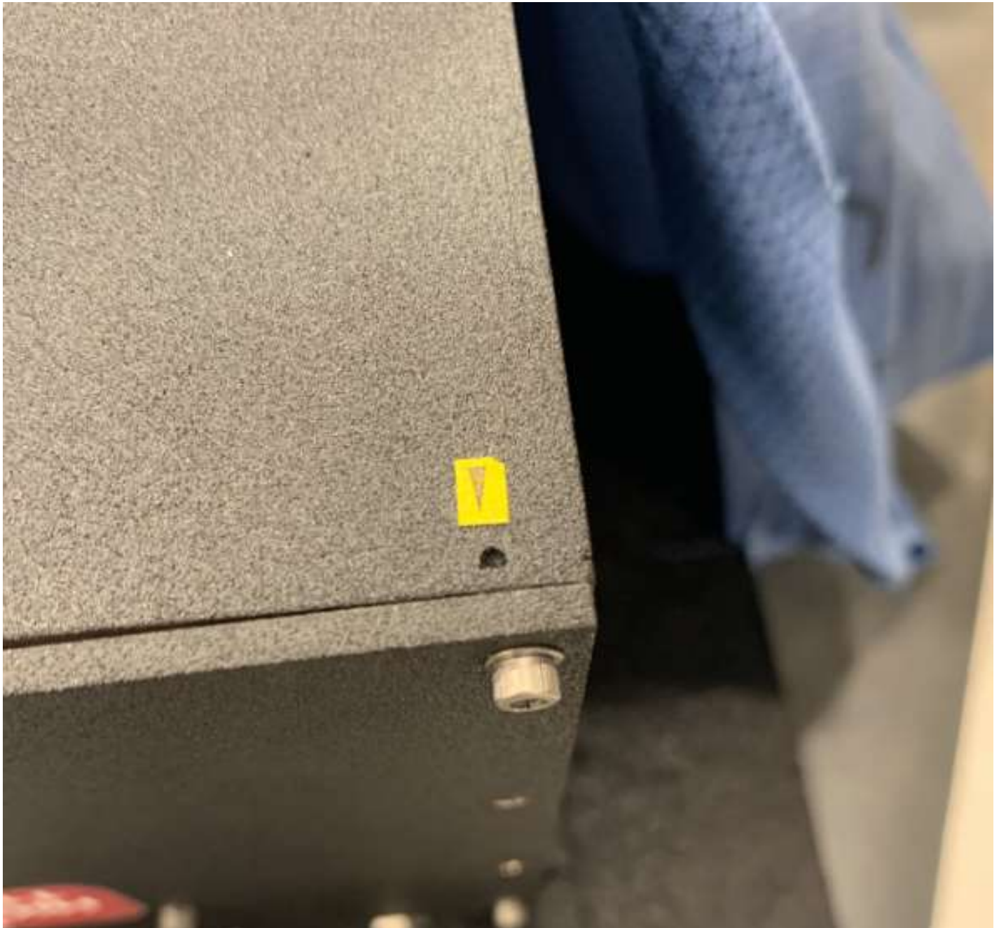
Figure 21: Example of a non-uniform powder-coated surface
