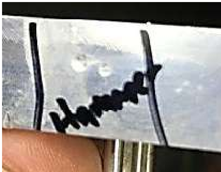
Figure 15: The above image shows damages from a hammer.
