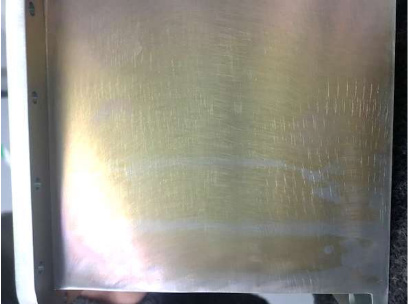
Figure 8: Notice the non-uniform color identified above. This is an example of poor coverage.
