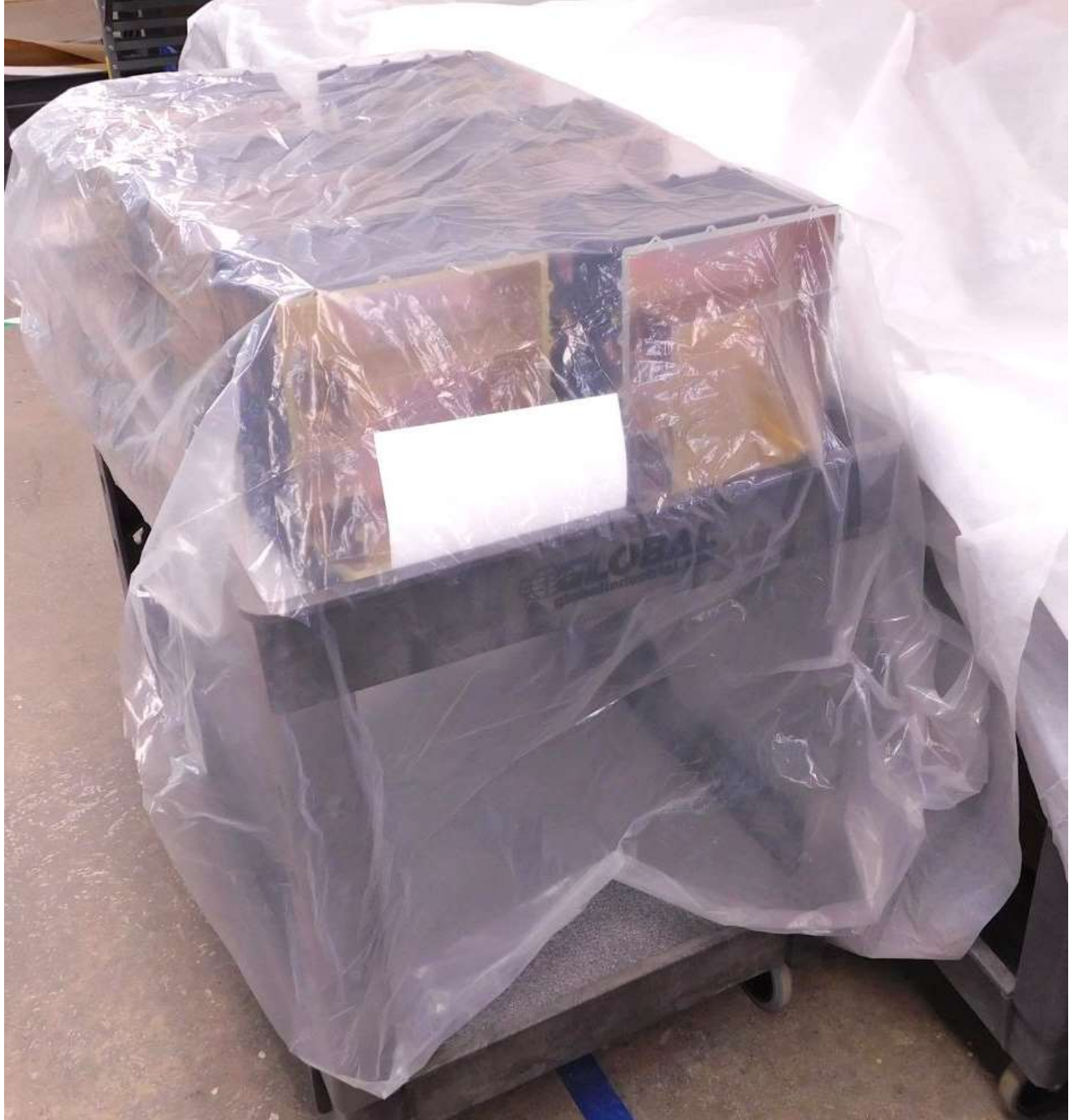
Figure 6: These parts are awaiting source inspection and have been properly covered to protect from FO/FOD contamination and damages.
