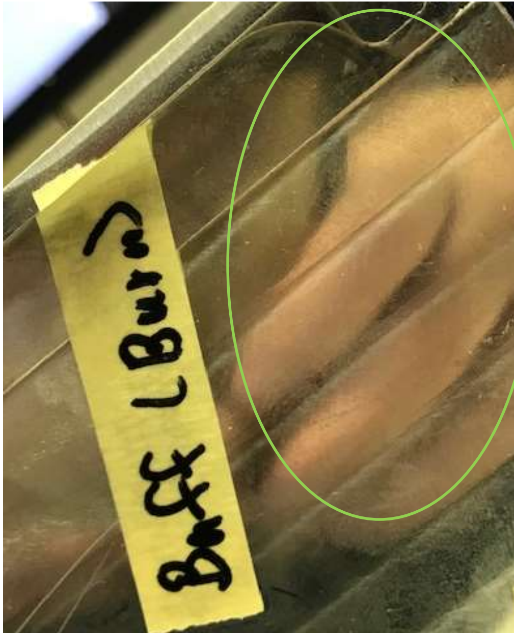
Figure 20: The faded area to the right of the tag (circled in green) shows over buffing known as a buff burn.
