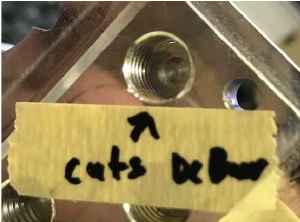
Figure 16: The above image shows damage from improper deburring around a threaded hole.
