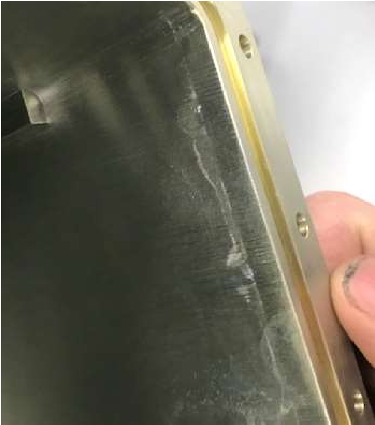
Figure 12: The white film on the braze seam is brazing salt residue. This improperly cleaned part had chemical conversion coating applied over top of the residue.
