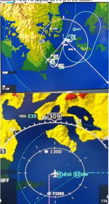
The mapped location of the airport itself is correct per the navigation database, but the surrounding terrain is rendering incorrectly.
