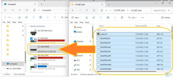
10. Navigate to the USB drive folder. You should see the new files that were created during the unzipping process of your databases. You can now remove your USB drive and proceed to upload your databases into your aircraft.
